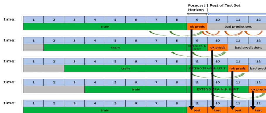
Fig. 1 Working principle of the rolling window mechanism
