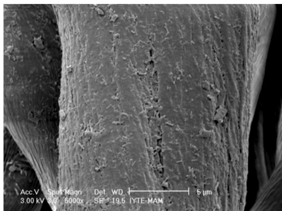
Figure 8. SEM photograph of argon plasma treated cotton sample under 130 W for 60 sec.
